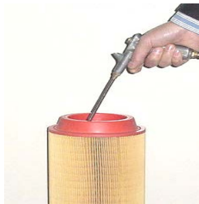
Figure 6-3 Air Filter Element Cleaning
