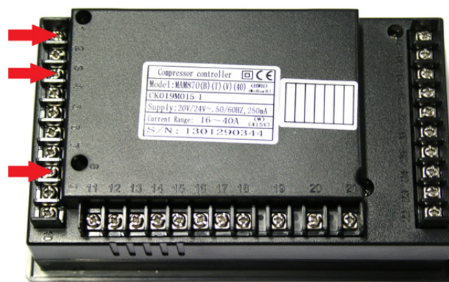
Figure B-1 Rear View of MAM-870 Controller
