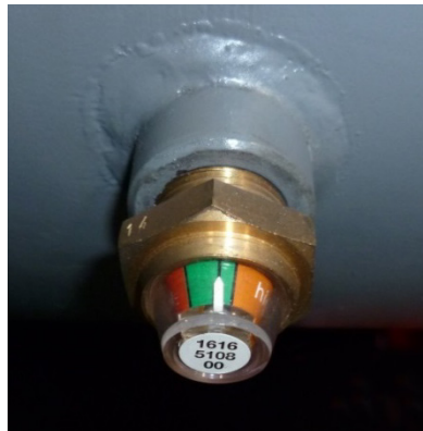
Figure 6-1 Full Oil Level Indication
