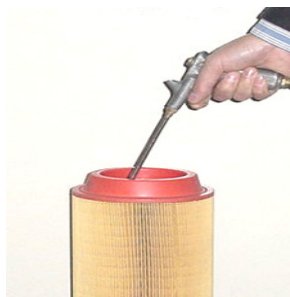
Figure 6-3 Air Filter Element Cleaning
