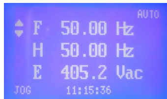
Figure B-3 VSD Display in AUTO Mode
