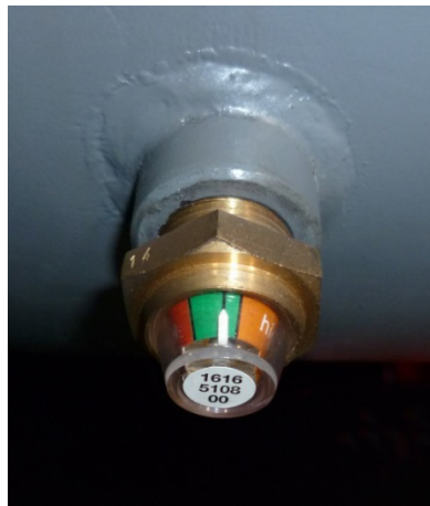
Figure 6-1 Full Oil Level Indication
