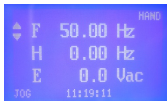
Figure B-4 VSD Display in HAND Mode
