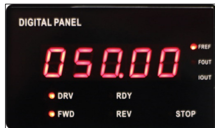
Figure B3 VSD Display in Running Mode
