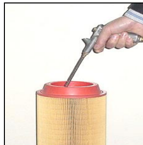
Figure 6-3 Air Filter Element Cleaning
