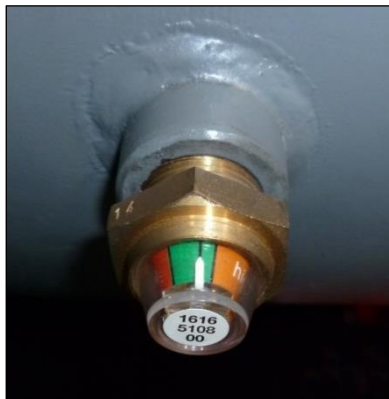
Figure 6-1 Full Oil Level Indication
