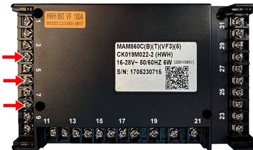
Figure C-1 Rear View of MAM-860 Controller
