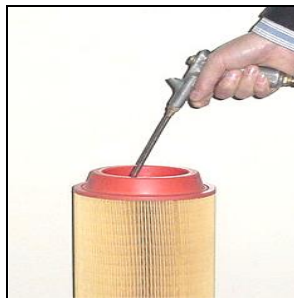
Figure 6-3 Air Filter Element Cleaning
