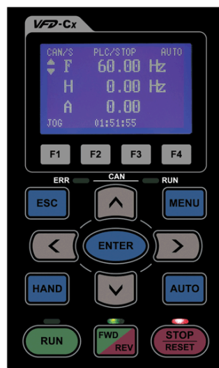
Figure B-2 Keypad and Display
