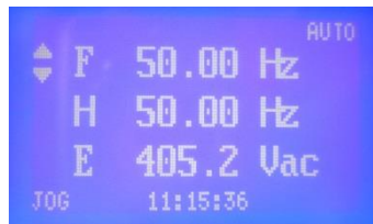
Figure B-3 VSD Display in AUTO Mode
