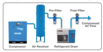
Senator Professional Packages satisfy the minimum essential requirements for compressed air production, storage and treatment in most industrial applications. Each package comprises an oil-lubricated compressor, receiver tank, refrigerant dryer and two stages of filtration. The clean, dry compressed air is suitable for pneumatic tools, air powered machinery, abrasive blasting, powder coating and spray painting.
