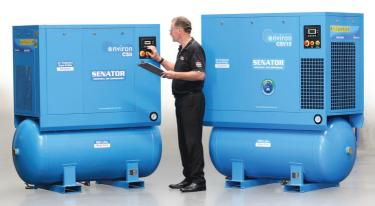
The Senator CS and CSV Series 4-in-1 compressed air stations comprise a rotary screw compressor, air receiver tank, refrigerant dryer and both pre- and post-filters in a single integrated package. Save on floor space and installation cost by choosing one of these ready-to-run units that will dependably provide your business with clean and dry compressed air.
