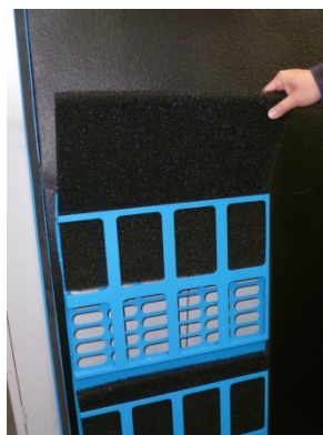
Figure 6-2 Air Pre-Filters Removal
