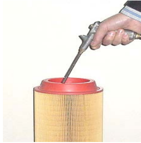
Figure 6-3 Air Filter Element Cleaning
