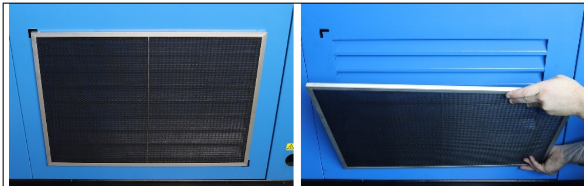
Figure 5-2: Air Pre-Filters Location and Removal
