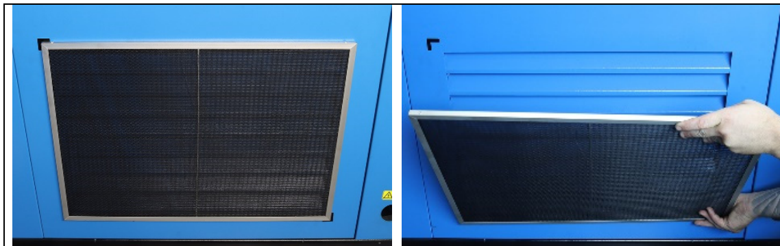
Figure 5-2: Air Pre-Filters Location and Removal
