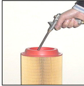
Figure 5-3: Air Filter Element Cleaning
