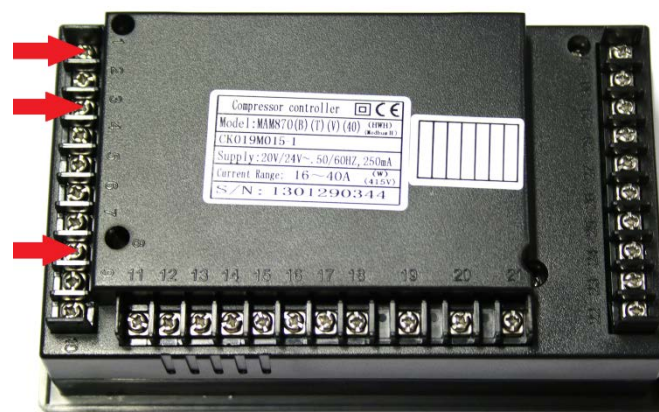
Figure B-1 Rear View of MAM-870 Controller
