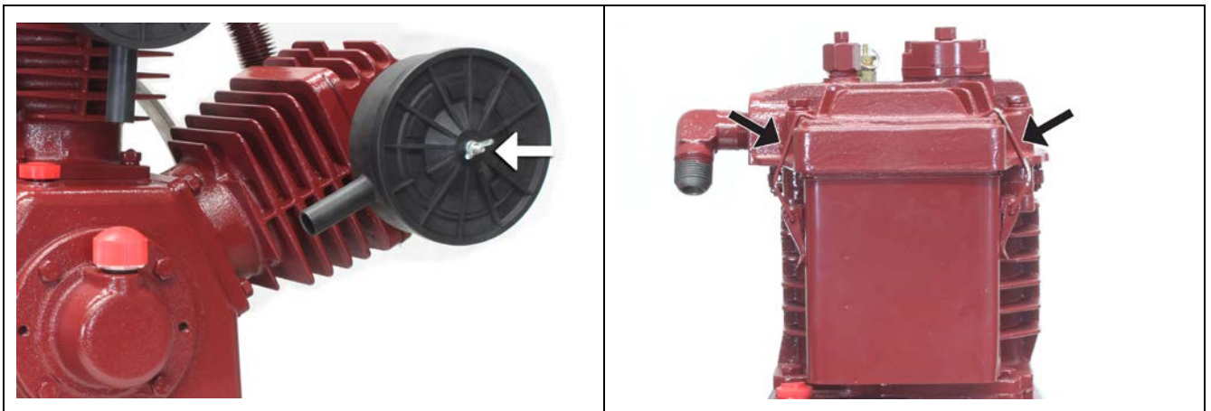
Figure 7-1 Air Filter Element Cover Removal – A-Series (L) and B-Series (R)
