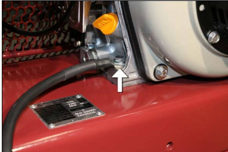
Figure 5-7 Battery Negative (-) Cable Connection to Engine Mounting Bolt
