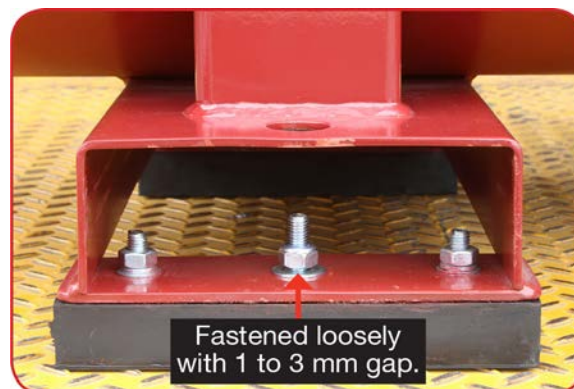
Figure 5-2 Basic Bolted-Down, Foot-Mounting Arrangement
